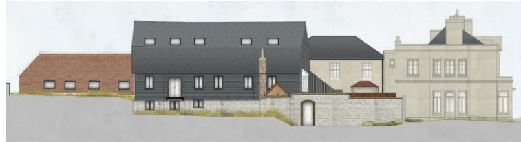
Fig. 6.20: Proposed south-west elevation of the barns and Manor House, showing the opening to the flint wall leading to the infill building.
